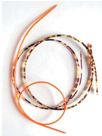
Figure 4. Non-celluloid rigid circulars — “amber” on the left and the very popular faux tortoiseshell on the right. These needles could not be used now, as they would break or crumble due to the disintegration of the chemical bonds over time.
