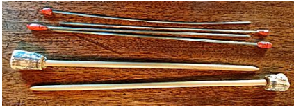
Figure 1. Double-pointed knitting needles with “caps” made of wax and cork. The wax examples here are very hard wax, so difficult to remove, essentially making these into single-point needles. But a softer wax could also be used, such as the bees wax included with sewing boxes to strengthen thread in the pre-mercerised days.
